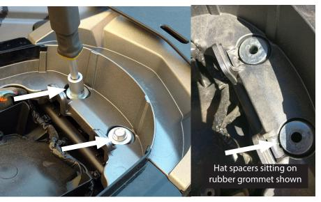
Use 12mm socket to remove the two M8 bolts as shown. The OEM hat spacers and rubber grommet that are below the washers stay and the bracket will mount on top.
