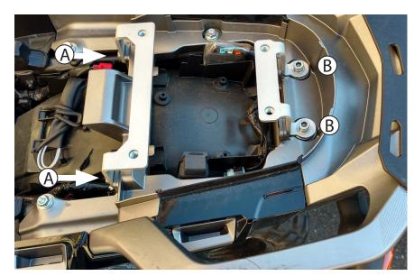
(A)Install front bracket as shown with OEM M6 hex screws from step 1.(B) Use M8 cap head screws with washers to install rear bracket as shown.
