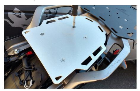
Use 5mm allen tool with M8 x 16mm flat head screws to install rack platform.
